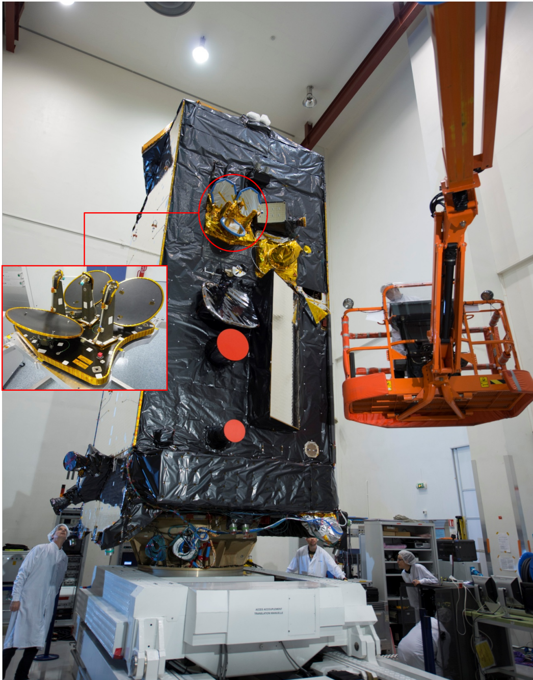
Figure 9: Alphasat satellite carrying the Q/V band technology demonstration payload.
