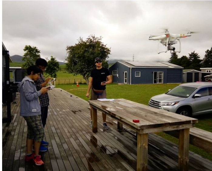
Figure 6: Measurement of the UAV energy consumption in the rural area of Rotorua, New Zealand. The data recorded during the experiment was used to tune the parameters used in our model.
